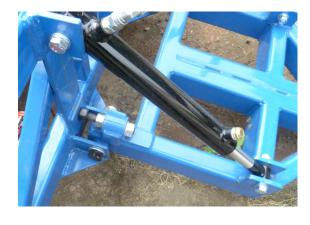
Lifting gear on Sweeper head for easy transportation
