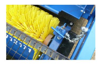
Easy brush adjustment allows collection of surface material or to scarify
